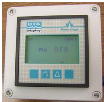
The screen will read "No DTS" when set up correctly
