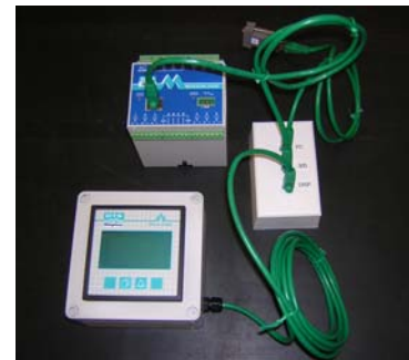
DTS-305 and DTS Portable Display Connected through a DI-001
