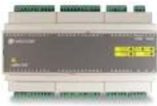
The **LM50-TCP+** is an instrument equipped with 50 voltage-free digital inputs. Through these inputs, using a master communications software, the user can detect the logical state of the inputs (open or closed contact), or otherwise know the number of impulses or manoeuvres received by an outside impulses emitter (energy, water, gas meter, etc). The recorded parameters are shown in the following variables table (see section 2.3.-).
