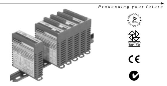
The Model 9004 is a miniature space saving 92 x 92 x 26 mm DIN-rail mount programmable load cell transmitter. Configuration and field calibration is done via a notebook or desktop PC using the user-friendly software available from our web site. Complete 3-way isolation is provided between power supply, input and output.
