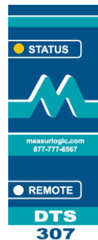
Orange – Energy is being generated/exported
