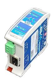
The DTS E4C family of Modbus Serial to Ethernet Gateways provides a bridge connection for devices on Modbus RS-485 Serial networks to communicate with Modbus TCP networks allowing for seamless integration.
