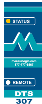
Orange – Energy is being generated/exported
